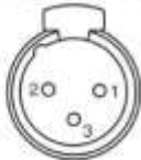
DMX - output XLR mounting-sockets (rear view):
