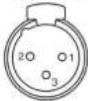
DMX - output XLR mounting-sockets (rear view):
